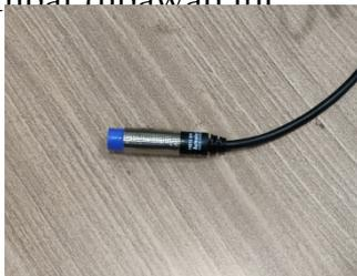
Gambar 11. Sensor *Autonics PRD12-8DN*
