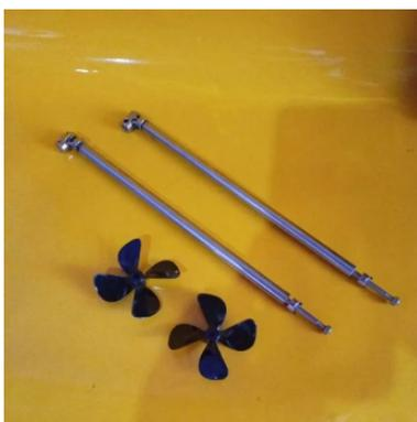
Gambar 4. Shaft propeller
